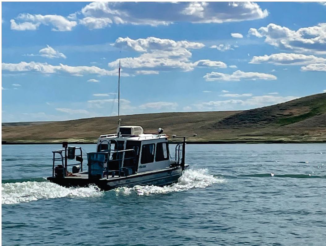
Figure A-2.—SeaArk boat with real-time kinematic Global Positioning System and multibeam depth sounder system.
