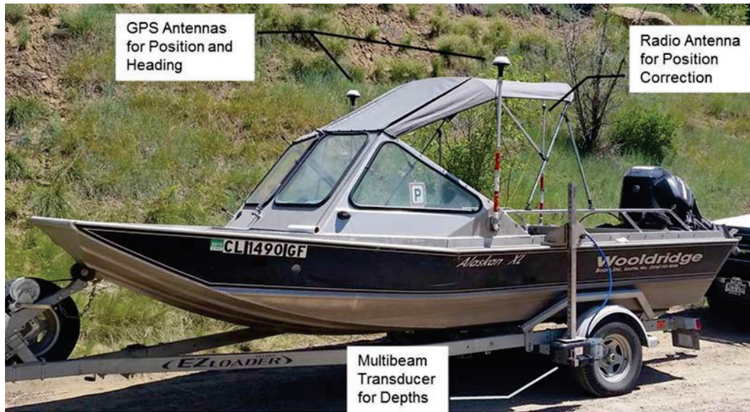
Figure A-1.—Wooldridge boat with real-time kinematic Global Positioning System and multibeam depth sounder system.
